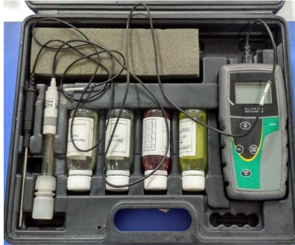
**Alat uji pH meter**
