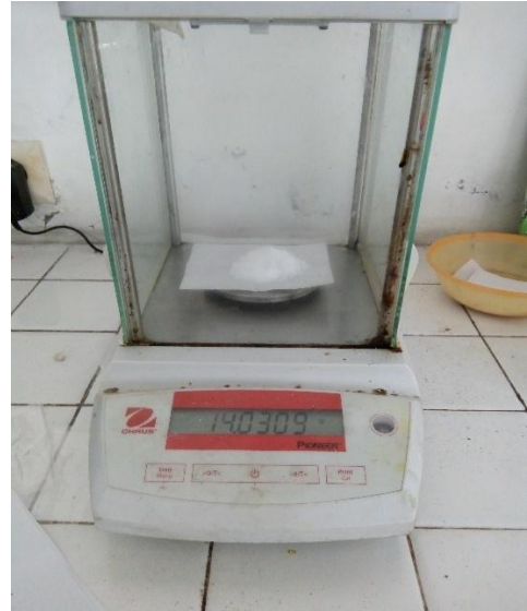
Gambar 2. Penimbangan Serbuk Kalsium klorida ( \text{CaCl}_2 )
