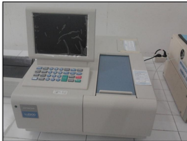
Spektrometer UV (HITACHI U-2900)
