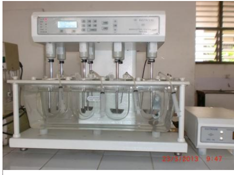
Dissolution tester tipe 2
