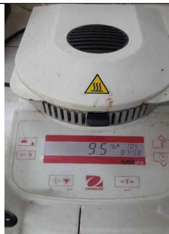
A photograph of a white digital food dryer. The digital display shows '9.5 %' and '105'. Below the display are several control buttons. A yellow warning label with a steam symbol is visible on the top left of the machine.  |
