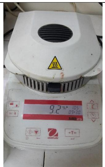
A photograph of a white digital food dryer. The digital display shows '9.2 %' and '105'. Below the display are several control buttons. A yellow warning label with a steam symbol is visible on the top left of the machine. |
