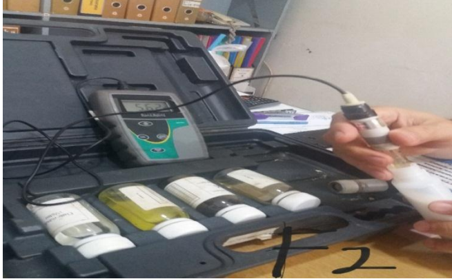
Pengujian pH losion pelembab VCO formula 2
