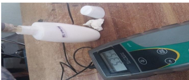
Pengujian pH losion pelembab VCO formula
