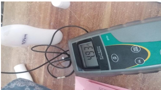
Pengujian pH losion pelembab VCO formula 4
