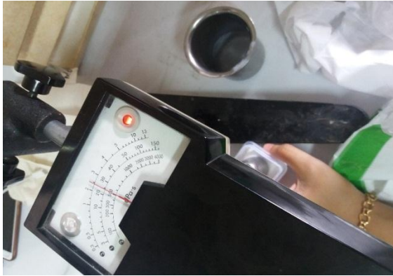
Pengujian viskositas losion pelembab VCO
