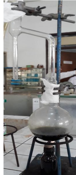
b. Gambar rangkaian alat Sterling Bidwell
