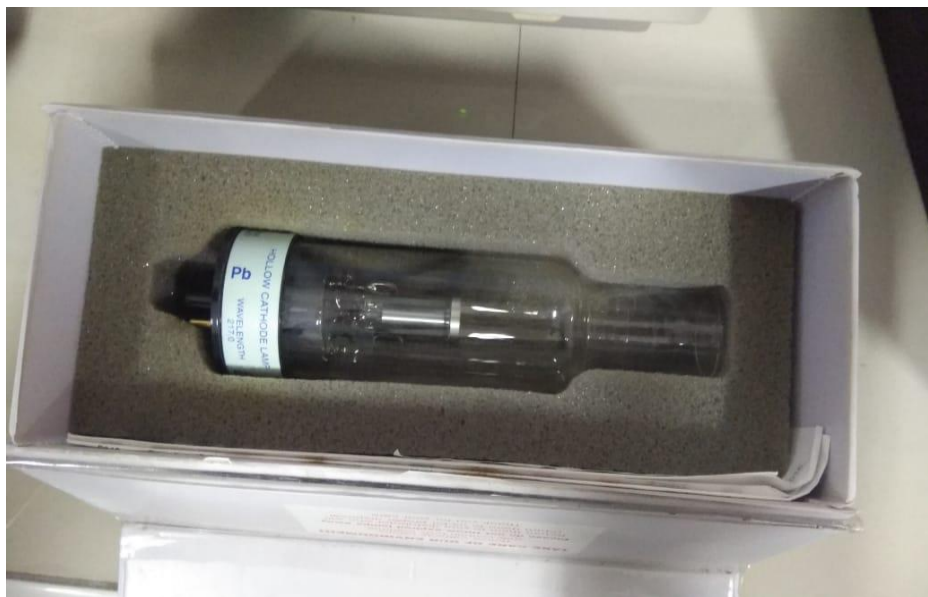
Gambar 2. Hellow Cathode Lamp Pb
