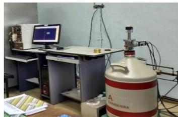
**Gambar 2.4. Rangkaian alat XRF (*X-Ray Fluorescence*)**
