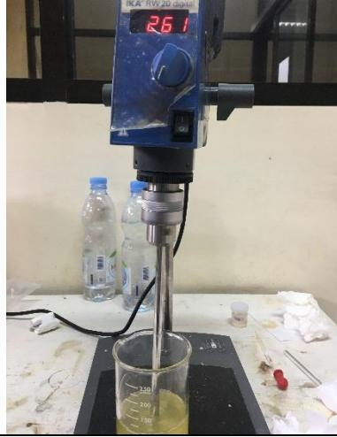
A photograph of a laboratory homogenizer. It features a blue motor unit with a digital display showing "251" and a black probe. The probe is inserted into a beaker filled with a yellowish substance, which is placed on a black hotplate. In the background, there are some water bottles and laboratory equipment. | Untuk mencampur dan menghomogenkan sediaan                              |
