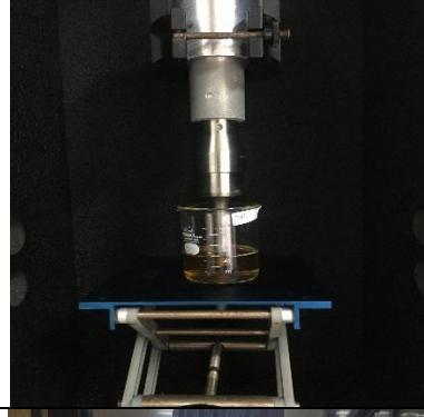
A photograph of a sonicator probe. It shows a metal probe submerged in a small beaker of liquid inside a dark, enclosed chamber.                                                                                                                                                                                       | Menghomogenkan dan memperkecil ukuran partikel                          |
