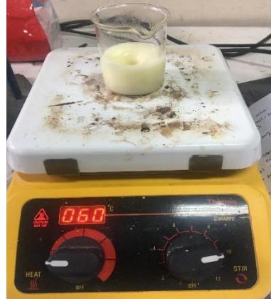
A photograph of a magnetic stirrer. It has a white top plate with a small glass beaker containing a yellowish liquid on it. Below the plate is a yellow control panel with a digital display showing "050" and two analog dials labeled "HEAT" and "STIR".                                                              | Untuk menghomogenkan suatu larutan dengan pengadukan menggunakan magnet |
