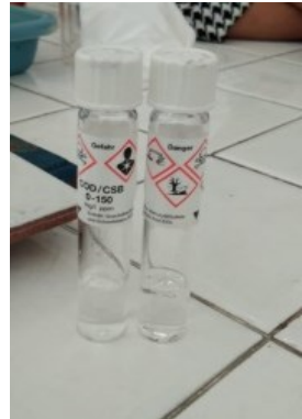
Gambar 19. Tube Digestion Vessel
