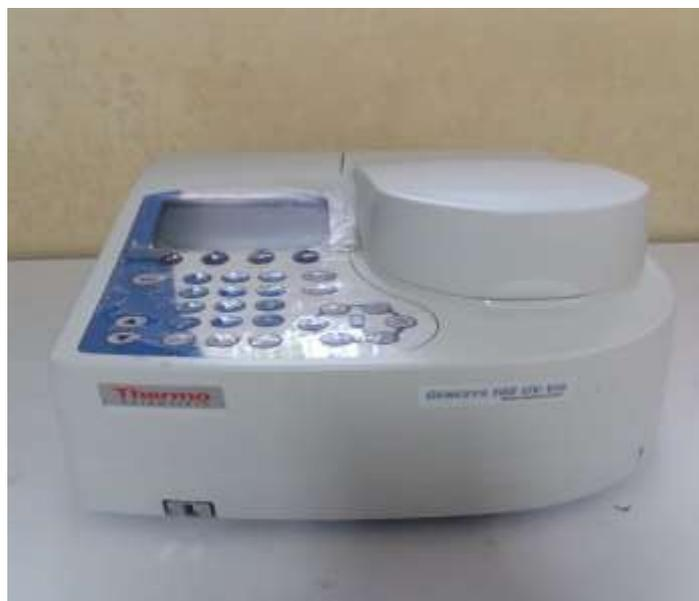
**Alat Spektrofotometri UV-Vis**
