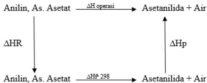
Gambar I-3 Diagram vektor  $\Delta H_{operasi}$
