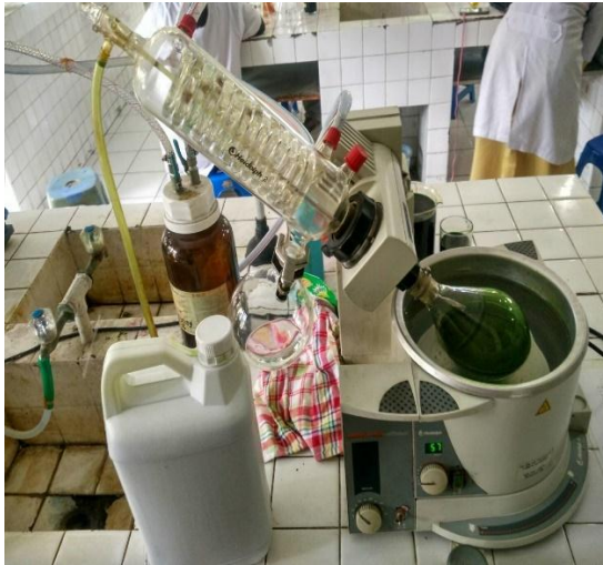
Evaporator daun pacar air
