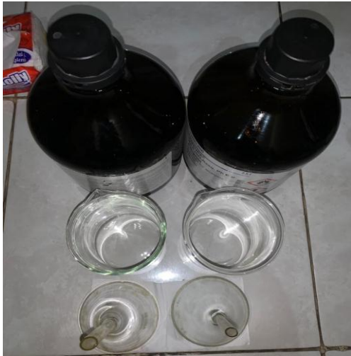
Alat maserasi (Maserator, beaker glass dan corong)
